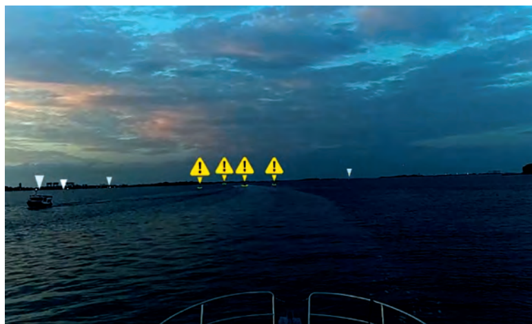
The Lookout camera system tracks objects in the water, using an AR view
