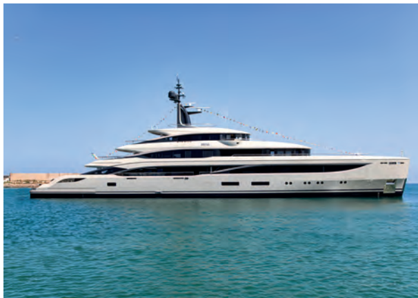
The six-deck Iryna has a range of 5,000nm at a cruise speed of 12knots
