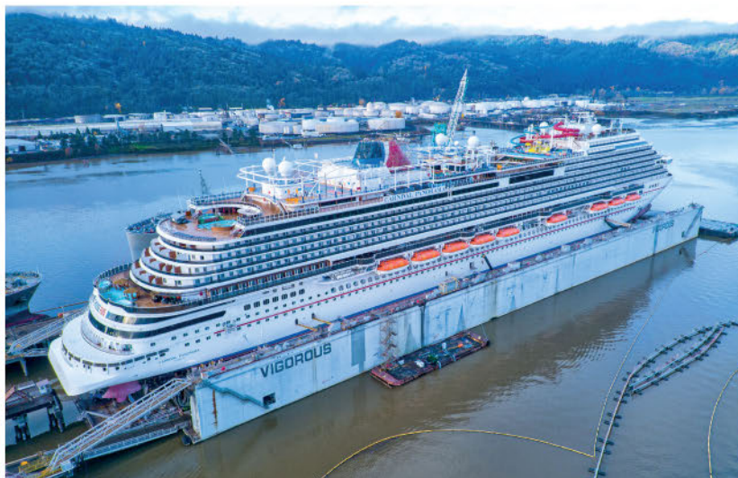
THE PORTLAND SHIPYARD'S FLOATING DOCK WAS USED FOR AN EMERGENCY REPAIR TO THE CRUISE SHIP CARNIVAL PANORAMA TOWARDS THE END OF LAST YEAR
