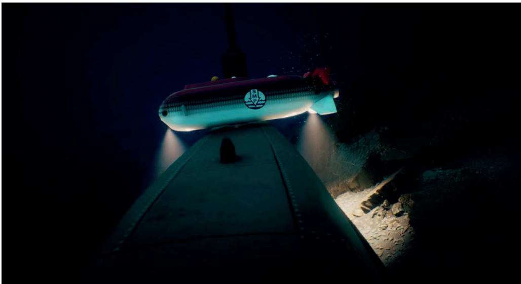
THE SRV-F MK3 IS A HYBRID SYSTEM CAPABLE OF DEPLOYMENT BY AIR AND ON A MOTHERSHIP
