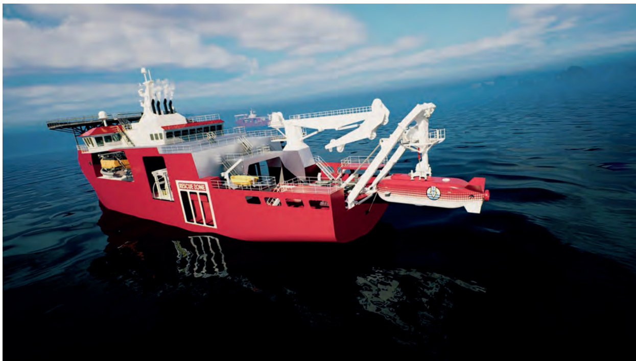
THE MOTHERSHIP DESIGNED BY HOULDER WILL HAVE A PERMANENT HYPERBARIC CHAMBER, 10-BERTH HOSPITAL AND ACCOMMODATION FOR UP TO 90 PEOPLE ALONG WITH SEPARATE ACCOMMODATION FOR RESCUED PERSONNEL
