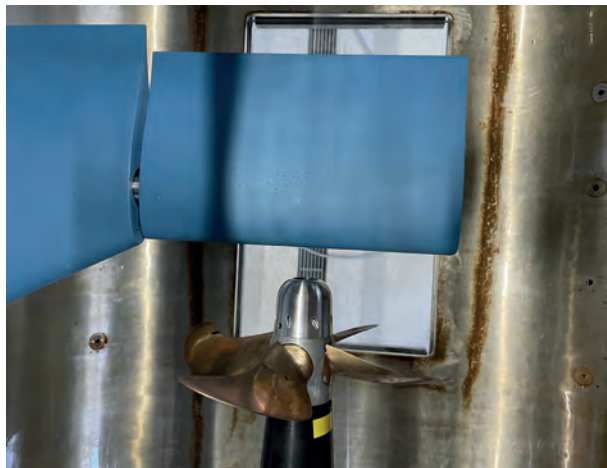
THE HOLY BOSS CAP HAS HOLES BORED INTO THE CONICALLY SHAPED HUB
