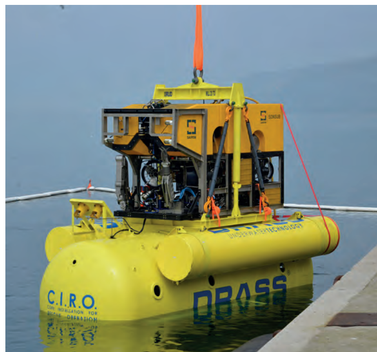
ARTIST'S IMPRESSION OF THE SUBMARINE RESCUE VEHICLE BASED ON THE DRASS RESCUE CAPSULE AND SAIPEM ROV
