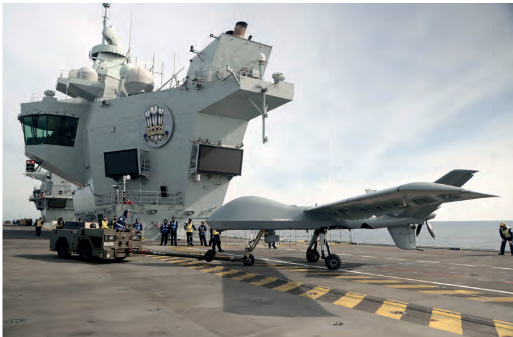
THE MOJAVE IS A VERSION OF THE MQ1C GRAY EAGLE AIRCRAFT ADAPTED FOR SHORT TAKE-OFF AND LANDING
