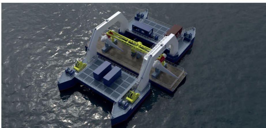
HydroWing's 41m loe Quad Hull Barge could reduce the cost of each wave turbine installation from £500,000 to £20,000
