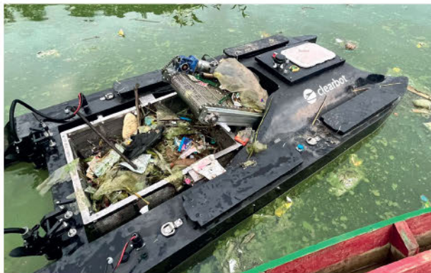
The battery-powered Clearbot is being used to tackle riverine pollution in India
