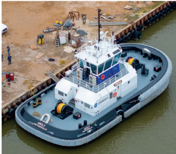
The US' first all-electric tug, eWolf , features a 6.2MWh Corvus Orca energy storage system
