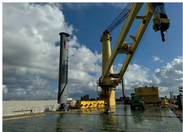
THE VENTOFOILS ARE MOUNTED ON A SPECIALLY DESIGNED FRAME THAT FACILITATES MOVEMENT ON THE DECK TO ACCOMMODATE PROJECT CARGO SHIPMENTS
