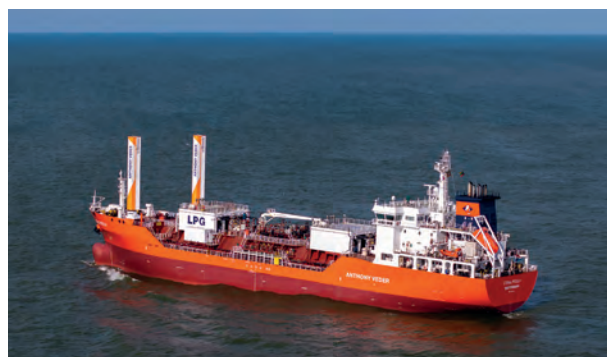
THE GAS CARRIER CORAL PATULA IS BELIEVED TO BE THE FIRST GAS CARRIER TO BE FITTED WITH A WIND ASSISTED PROPULSION SYSTEM
