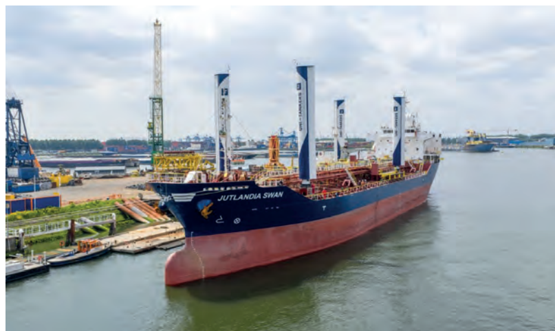
Chemical tanker Jutlandia Swan has been retrofitted with four Econowind VentoFoil
