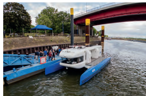
NOVA features 320kWh of battery capacity
