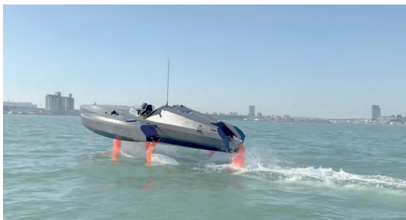
The prototype could provide the basis for a 24m foiling ferry, capable of speeds of 26-28 knots
