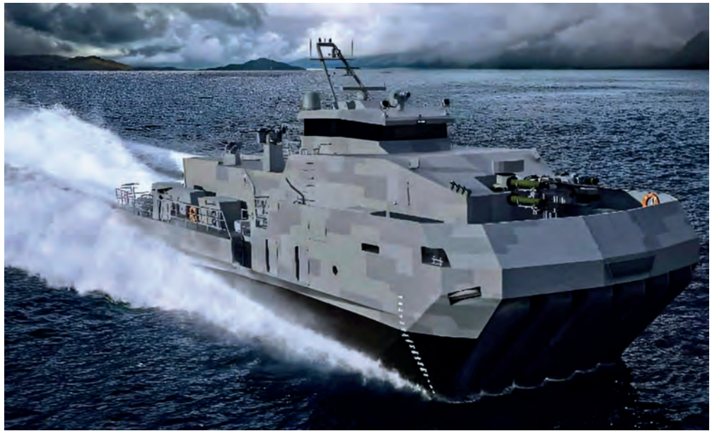
The design of the Aircat Bengal MC is an interesting combination of SES technology and autonomy
