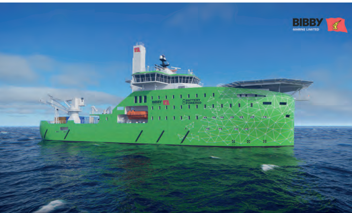
The eCSOV concept has a range exceeding 130nm on battery power alone
