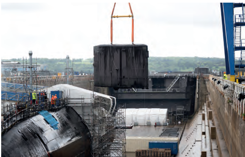
Removal of the fin from Swiftsure was an important milestone in the submarine dismantling project
