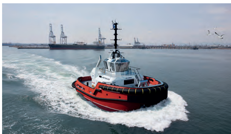
The ASD Tug 2312 series has a bollard pull of 70tonnes ahead
