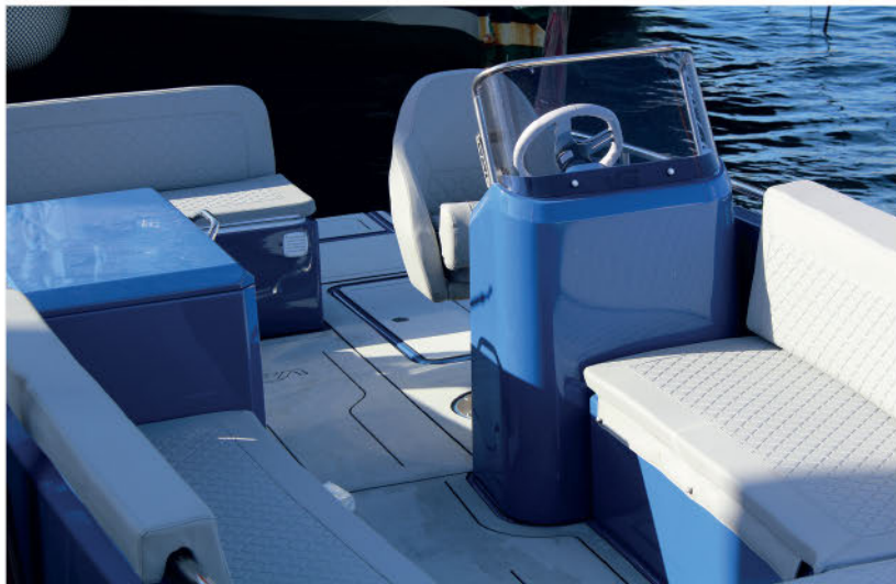
About 99% of the polypropylene boat was produced in a single piece, minus some smaller components
