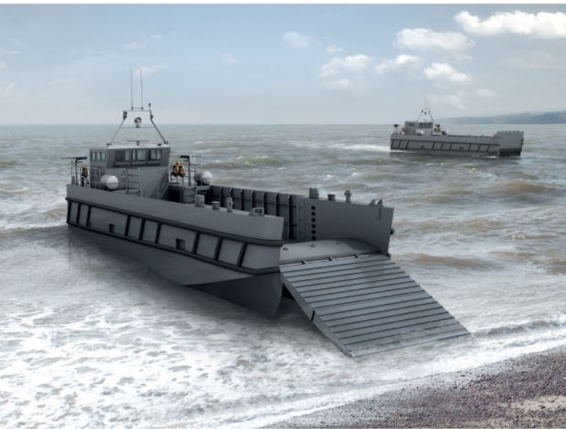
The Caimen series ranges from the Caimen-60 (pictured), with 60tonne capacity for payload and fuel, to the somewhat larger Caimen-150
