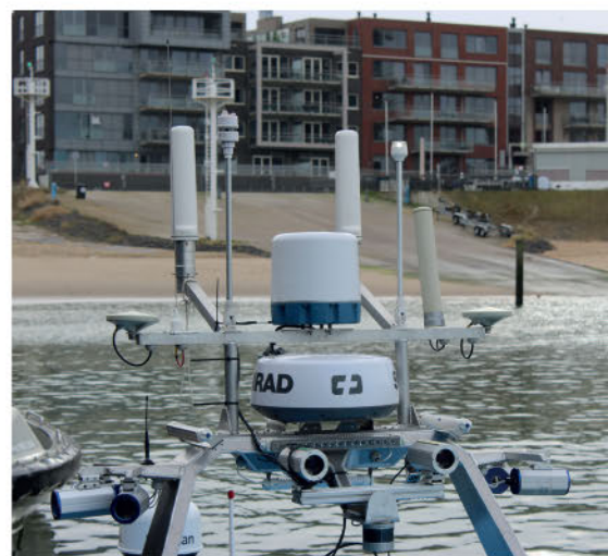
The MAS10 radar was developed with autonomous and uncrewed vessels in mind
