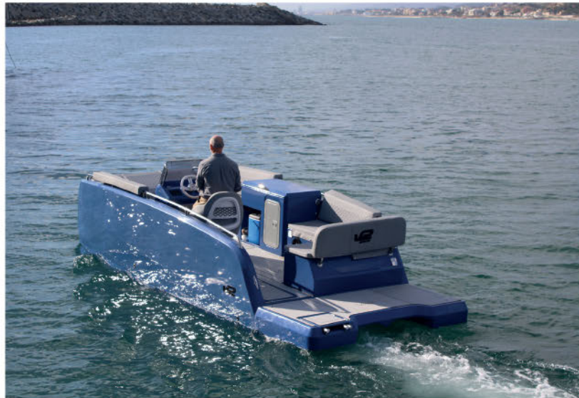
The 6m x 2.26m AM Cat runs on batteries feeding an 11kW electric motor
