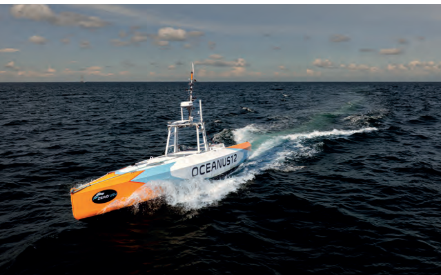
The company's Oceanus12 is designed for 20-day missions, but a forthcoming 'extra-long-range' version could up this to more than 60 days
