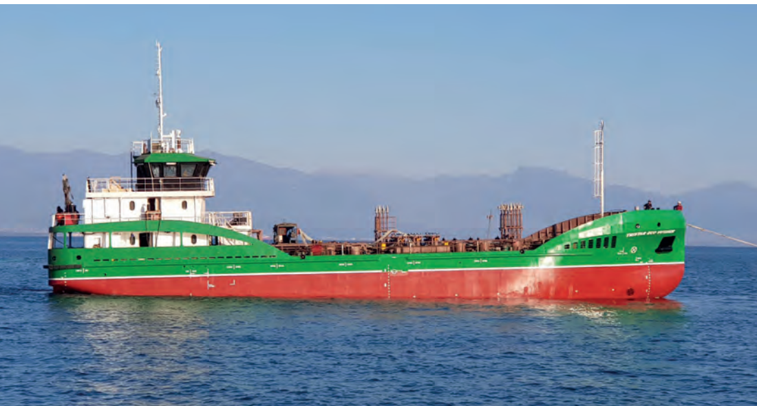
The new hybrid tanker can run on MGO, biofuel or battery power (image: Akdeniz Shipyard)
