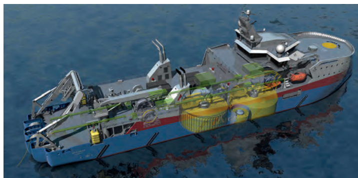
The 8,200dwt CLV will feature a cable capacity of 5,500tonnes
