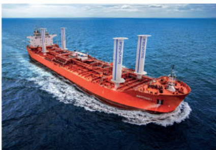
THE SUCTION SAIL TECHNOLOGY WILL BE INSTALLED ON SANTIAGO I IN 2025. SOURCE: BOUND4BLUE
