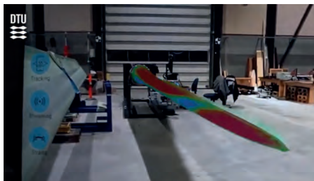
FIGURE 7. SIMCENTER 3D SMART VIRTUAL SENSING COMBINED WITH THE MODAL ANALYSIS OF A WIND TURBINE BLADE (COURTESY OF DTU)
