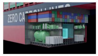
HEC/ABS CONCEPT ARRANGEMENT OF NUCLEAR REACTOR AND SUPPORTING EQUIPMENT. SOURCE: ABS
