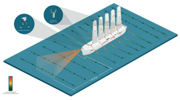
ULTRASONIC ANEMOMETERS COMBINED WITH THE WIND LIDAR IMPROVE THE ACCURACY OF WIND DATA IN WASP SYSTEMS
