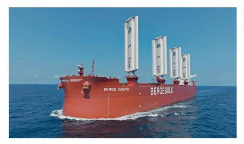
BERGE BULK'S BERGE OLYMPUS WITH FOUR 37.5M WINDWINGS DEPLOYED
