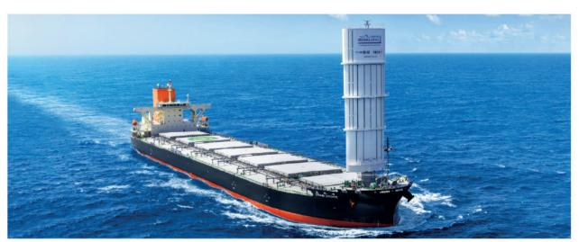
MOL HAS CONTINUOUSLY MEASURED THE PERFORMANCE OF ITS PROPRIETARY WIND CHALLENGER SYSTEM ON BULKER SHOFU MARU SINCE ITS DELIVERY IN OCTOBER 2022, CONFIRMING FUEL SAVINGS OF UP TO 17% ON ITS VOYAGES. THE COMPANY PLANS TO LAUNCH 25 VESSELS EQUIPPED WITH THE SYSTEM BY 2030, SOURCE: MOL
