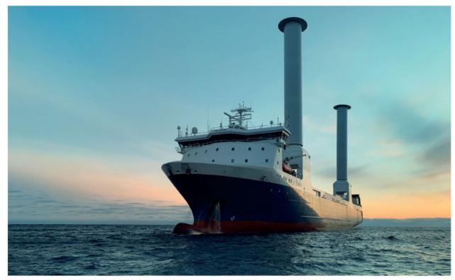
SEA-CARGO AS'S SC CONNECTOR RO-RO VESSEL EQUIPPED WITH NORSEPOWER ROTOR SAILS. SOURCE: NORSEPOWER
