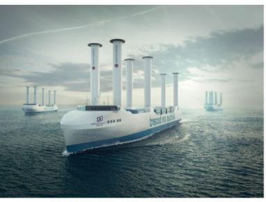
EACH OF LDA'S NEWBUILD RO-RO VESSELS WILL BE POWERED BY A COMBINATION OF SIX FLETTNER ROTORS, SOURCE: LDA
