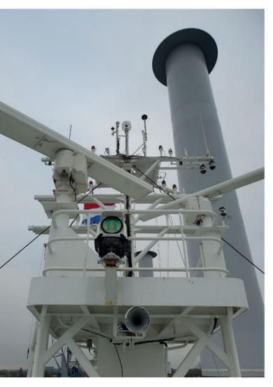
The implications of this collaboration are far-reaching. By comparing the LiDAR data with the rotor sail's thrust measurements, Norsepower can fine-tune its control systems, ensuring optimal performance in various wind conditions. This level of precision not only enhances the energy efficiency of vessels equipped with rotor sails but also significantly contributes to maritime industrywide decarbonisation goals.
