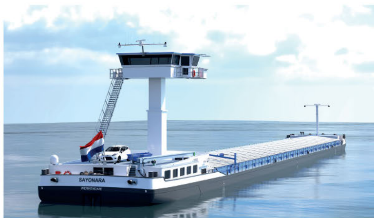
THE HULL SHAPE OF THE CDS DRY CARGO 110 VESSELS IS BASED ON THE PARSIFAL TYPE TANKER. SOURCE: CONCORDIA DAMEN
