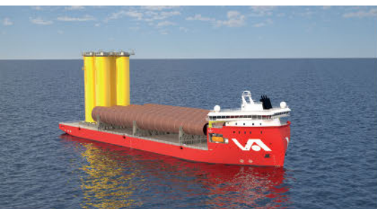
THE NEW VESSEL WILL FEATURE DUAL-FUEL ENGINES AND A BATTERY ENERGY STORAGE SYSTEM
