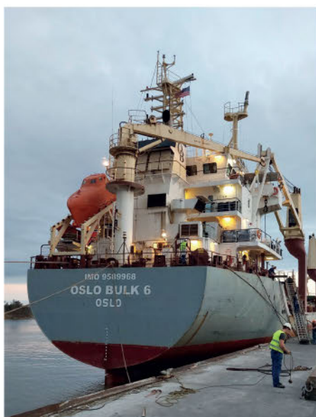
AN ASSESSMENT ON OSLO BULK 6 INDICATED THAT EEXI NEEDS WOULD BE SATISFIED BY DERATING ITS MAIN ENGINE TO COMPLY WITH THE NEW REGULATIONS
