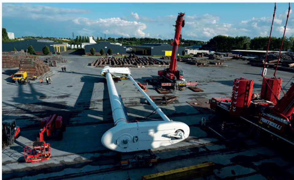
THE OCEANWINGS 363 ON THE RO-RO ARE 11M WIDE AND 37M HIGH. © JIFMAR GROUP LIBRARY/MADFLY - Y. DERENNE
