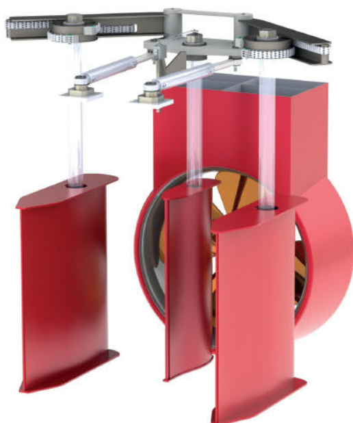
VAN DER VELDEN THREE-RUDDER SYSTEM. SOURCE: DMC
