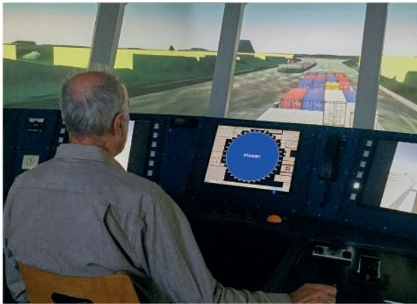
FIGURE 5. TWO SKIPPERS PERFORMING A MEETING MANOEUVRE ON COUPLED FULL MISSION BRIDGE SIMULATORS AT FHR. THE PHOTO ON THE RIGHT WAS TAKEN 20 SECONDS AFTER THE PHOTO ON THE LEFT
